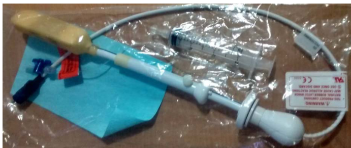
[Table/Fig-1]: Endorectal MRI coil.
